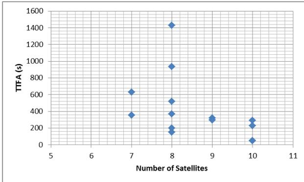
**Figure 10 – Short Baseline: TTFA vs number of visible satellites**
